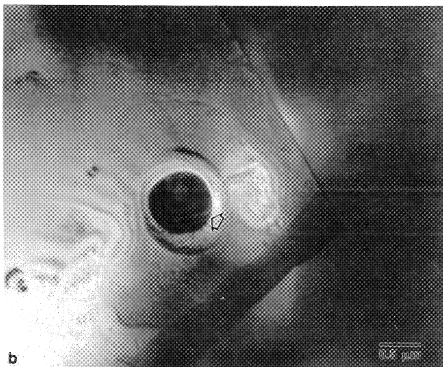
Fig. 15—(a) X-ray spectrum and (b) Bright-field electron micrograph of Ti(W)-carbides located within grain interiors of the HP-TiC material.
